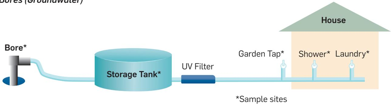
The intake (bore) is an important part of your system. Usually, providing a good intake is only a little more expensive than a poor one, yet a good intake will fix many of the problems caused by turbidity and other contaminants.
